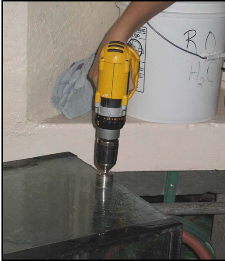
Figure 4. Demonstration of how to drill a hole in a glass aquarium using a diamond-tipped drill bit. Photographed at the AZA Amphibian Biology and Management School where everyone gets to try their hand at drilling a tank. (Photo: J. Pramuk)
