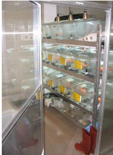
Figure 9. Lighting accommodated into the racks.
